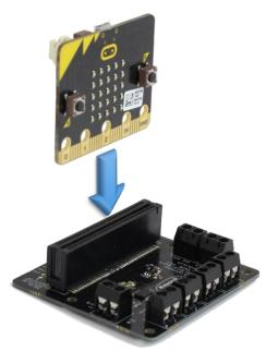
Inserting a BBC micro:bit: To use the motor driver board the BBC micro:bit should be inserted firmly into the connector as shown left.
